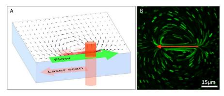
**A:** Principle of the method: Moderate heating of the sample with a rapidly scanned infrared laser induces directional thermo-viscous fluid flows. By flexibly designing the scan pattern of the laser, the fluid is pumped along pre-defined paths in the focal plane of the microscope. **B:** Transport of fluorescence beads: The red arrow indicates the scan direction of the focused infrared laser.
